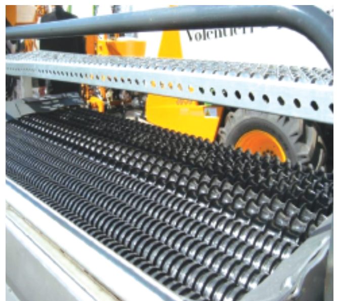
Fig. 27 - Detail of the new Pellenc Selectiv' Process harvestinghead. In particular, it highlighted high frequency linear destemmer (a) and the roller drive sorting table (b).
